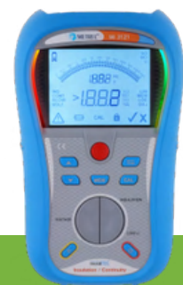
Brand: METREL Model: MI 3123 Use: Earth Resistance
