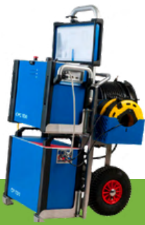
Brand: Omicron Model: CPC 100 & CP TD 1 Use: Primary Test System & Transformer Diagnosis
